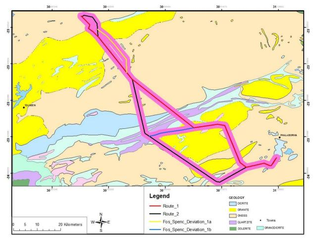
Fig. 7. Geology under the two proposed powerline routes.
